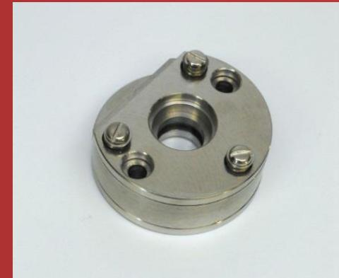
The IR cell path length need to be verified regularly, frequency depending of the type of products analyzed, since it may change over time due gradual erosion of the cell internal surface (1% per month, up to 12% per year)
